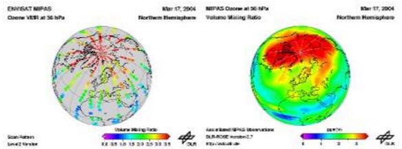
Figure 2. Example for ozone observations on a single day measured from the ENVISAT/MIPAS instrument (left) and a corresponding, assimilated ozone distribution for the respective day (right) derived with the DLR-ROSE model (Courtesy of DLR-DFD, Dr. Michael Bittner and Dr. Thilo Ebertseder).
